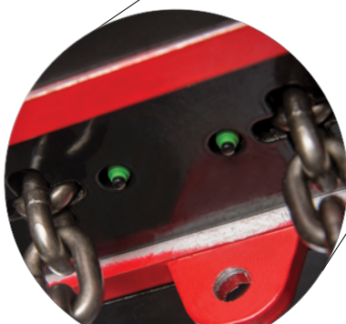
Upper and lower limit micro switch
