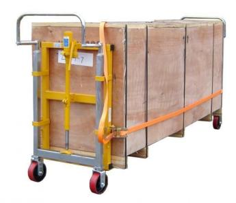
The cabinet being transported must not be left unattended standing on the equipment; it must always be lowered onto the floor. The securing straps may only be opened when the cabinet being transported, or the platforms, is standing on the floor. Never use this equipment for towing behind a vehicle.
