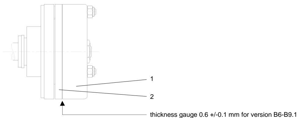
figure 31: adjusting the brake B6-B9.1
