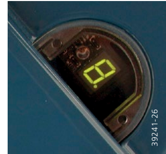
Display for elapsed operating time counter and operating statuses
